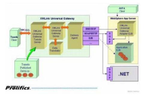
Figure 2-1 XMLink Universal Gateway Components
