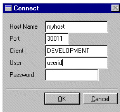
Figure 9-2 Connect to the middleware for a client not on a server machine, also called a remote client.
