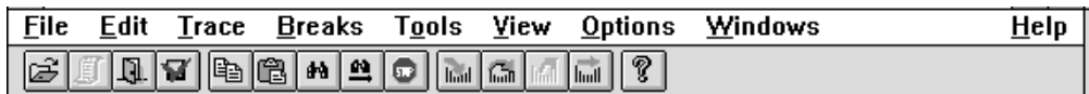
Figure 39-4 The debugger menu bar includes a Tools menu option when the debugger is run in expert mode.
